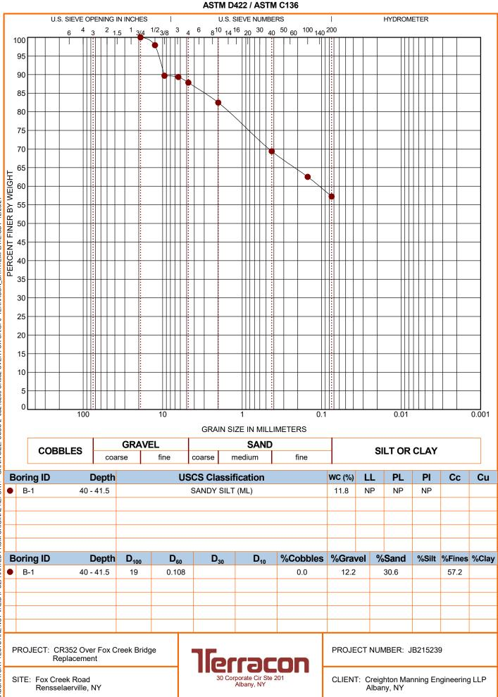
GRAIN SIZE: USCS-2 JB215239 CR352 OVER FOX CR.GPJ TERRACON DATATEMPLATE.GDT 12/28/21 LABORATORY TESTS ARE NOT VALID IF SEPARATED FROM ORIGINAL REPORT.
